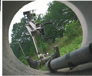
2. The iRobot 510 PackBot has a number of built-in cameras, along with mounting points for more specialized cameras and sensors.
